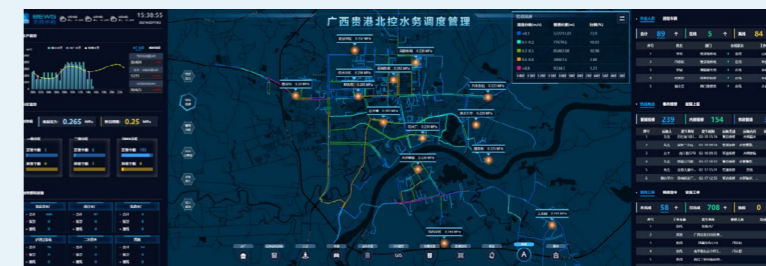
Comprehensive intelligent water distribution control platform
